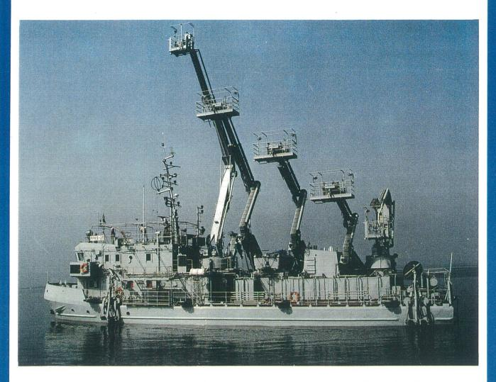
The ship – painting station is intended for cleaning and painting of the external surfaces of war and merchant ships, and for underwater cleaning of the hull fouling.
